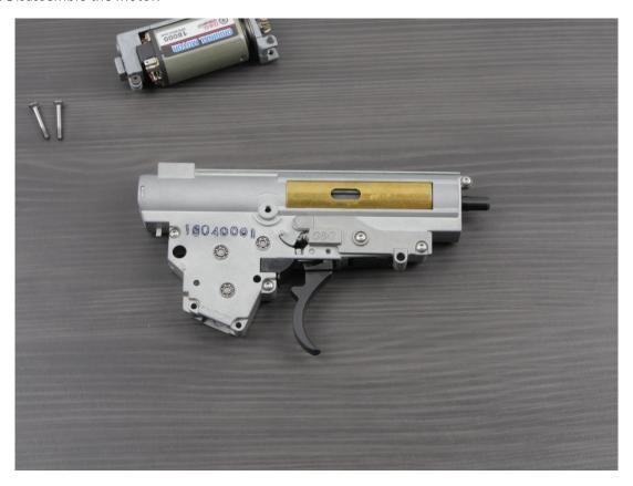
1.2. Dismantle the gearbox external parts (sector gear cover, trigger lock, screws).
