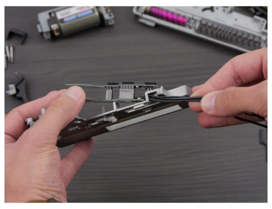
2.3 Carefully place the bottom board in the gearbox shell. **TITAN V3 fits CNC gearboxes with very small** backlash. While fitting TITAN, pull cables and at the same time push board in to right place.
