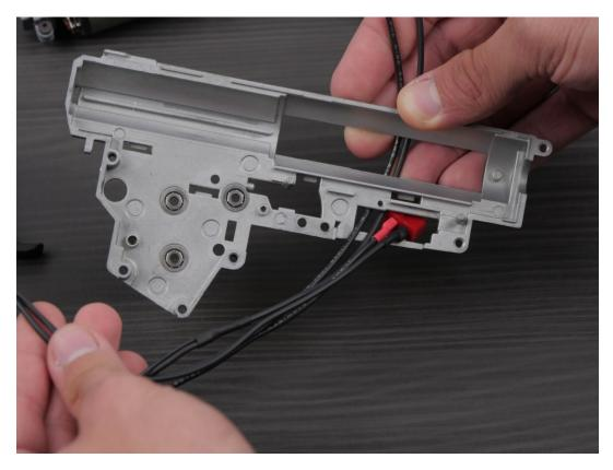
2.2 Place the wires in gearbox shell so as the unit can fit properly without any resistance.
