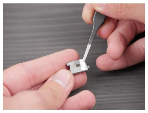
4.3 Paste one Trigger anti-backlash sticker inside the moving element of the trigger.
